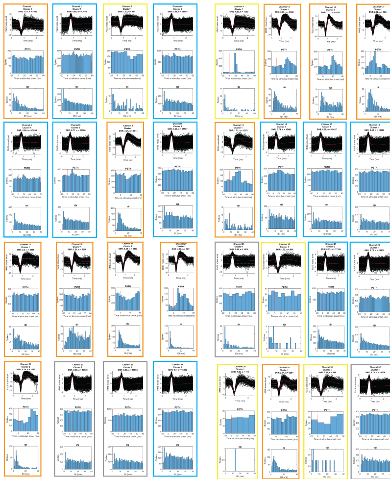
Figure B2: Summary of data recorded from Cat 2 by an N-Form 3D microelectrode. Orange border signifies a single unit or potential multi-unit recording, yellow border signifies evidence of multi-unit recording, blue border signifies a functioning site based upon RMS noise level, and grey border signifies a site of indeterminate functionality.
